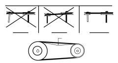
FIGURE 8: PULLEY ALIGNMENT & TENSION
